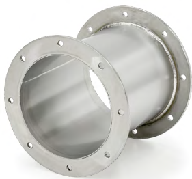
Welded tube V2A (1.4301) with welded flat flanges as per DIN 24154 R2
